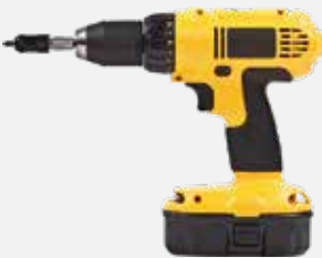
Cordless Drill To install screws and drill pilot holes as needed
