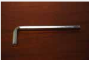
Allen Wrench For tightening bottom bolt Size: 5 mm Wrench
